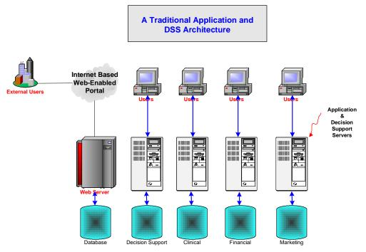
Figure 2 A Traditional Architecture Lacking Integration of Databases
